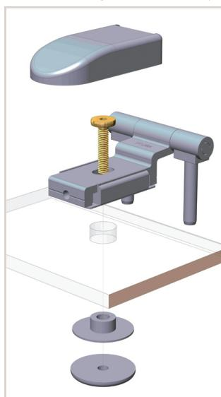
10. Attach the topmost frame screw on the lock side. Check the straightness of the corners with carpenter's square/spirit level. Check the openings by closing the door.
